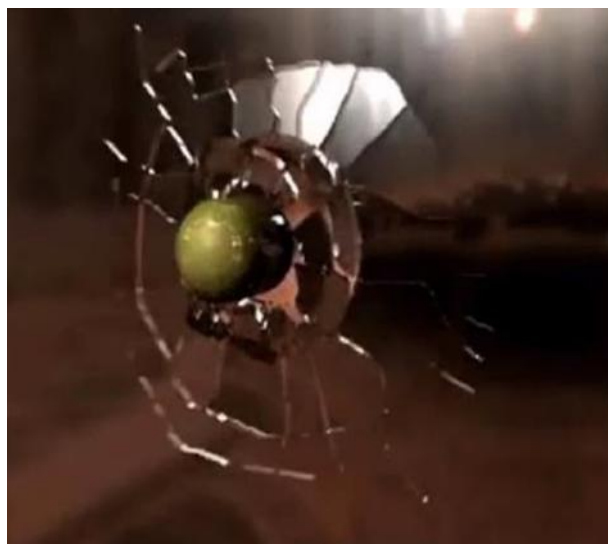
FIGURE-7: RADIAL AND CONCENTRIC FRACTURES IN GLASS FRACTURES
