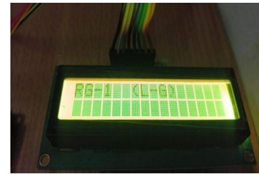
FIG. 2: TYPES OF FAULTS DISPLAYING ON LCD.
