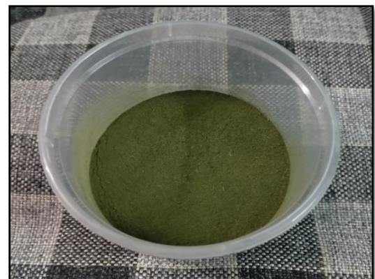
FIG.5 BIOMASS OBTAINED AFTER OVEN DRYING FOR ABOUT 4- 5 HRS
