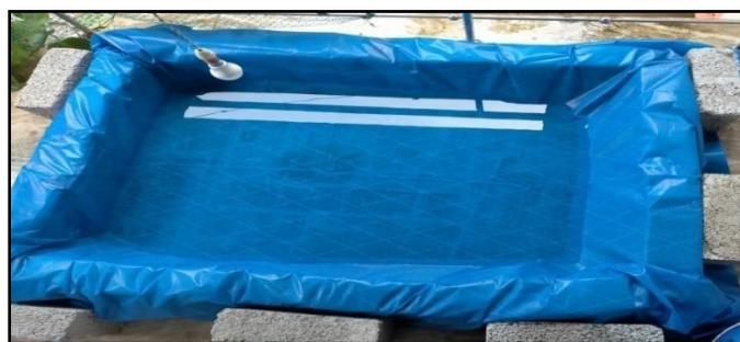
FIG.2 LAYER OF BRICKS COVERED USING TARPAULIN SHEET
