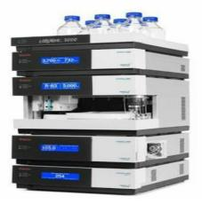
In nano-LC, the conventional instrumentation is all miniaturized. Pumps, connections. Columns, injection loop and detection interface are dimensioned for small volumes and low backpressure. These parameters can greatly influence the chromatographic efficiency of nano-LC and need to be controlled for a successful separation.
