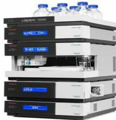
In nano-LC, the conventional instrumentation is all miniaturized. Pumps, connections. Columns, injection loop and detection interface are dimensioned for small volumes and low backpressure. These parameters can greatly influence the chromatographic efficiency of nano-LC and need to be controlled for a successful separation.
