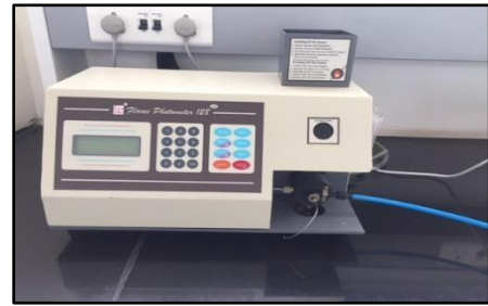
FIG. 14 THE FLAME PHOTOMETER USED TO DETERMINE THE POTASSIUM CONTENT
