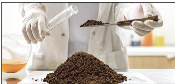
FIG. 13 THE LABORATORY TREATMENT OF THE COMPOST FOR THE ESTIMATION OF PHOSPHORUS CONTENT
