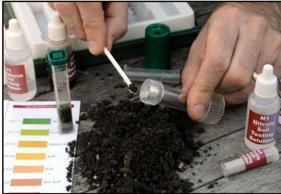
FIG. 12 THE TESTS CARRIED OUT TO DETERMINE THE PH OF THE MANURE IS SHOWN IN THE FIGURE
