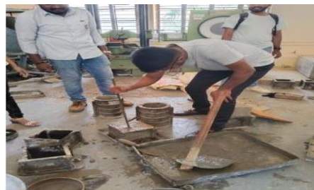
Fig. 1 - (a) compacting of concrete
