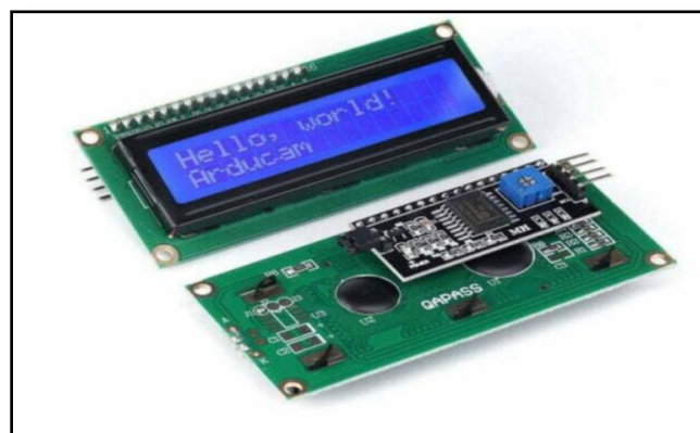
FIG 3. LCD DISPLAY(16X2) WITH I2C
