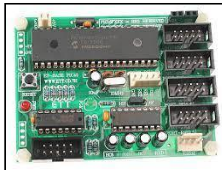
FIG-4 PIC CONTROLLER
