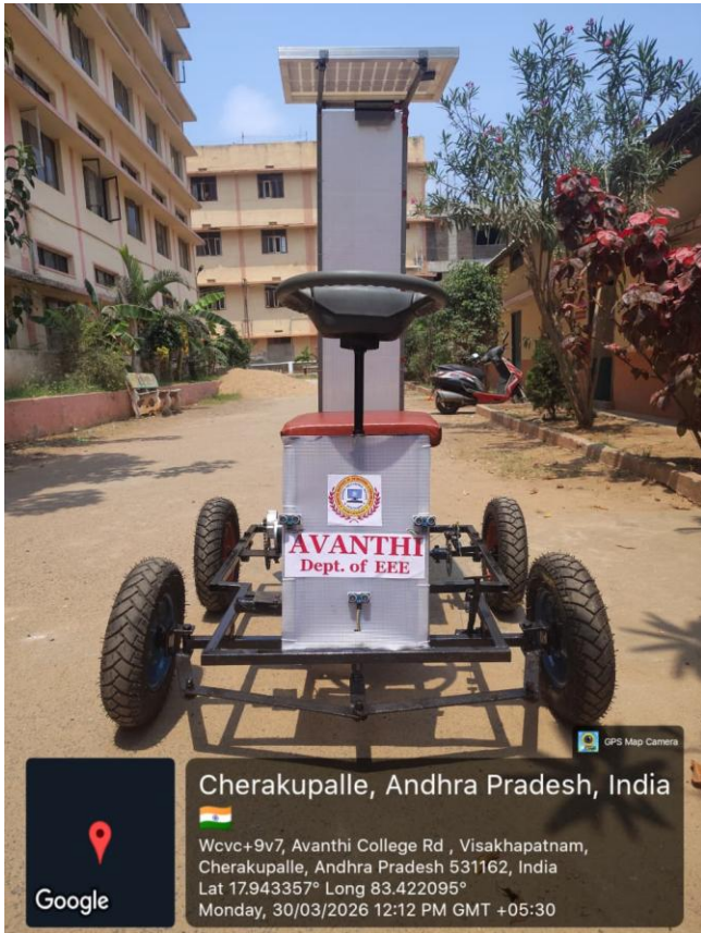
FIG. 1: FABRICATED FOUR-WHEELED ELECTRIC VEHICLE USING BLDC MOTOR
